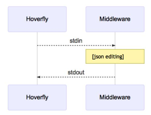
Hoverfly will send the JSON object to middleware via the standard input stream. Hoverfly will then listen to the standard output stream and wait for the JSON object to be returned.
