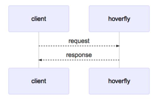
**Note:** When running as a webserver, Hoverfly cannot capture traffic (see *Capture mode*) - it can only be used to simulate and synthesize APIs (see *Simulate mode* and *Synthesize mode*). For this reason, when you use Hoverfly as a webserver, you should have Hoverfly simulations ready to be loaded.
