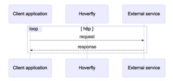
In Capture mode, Hoverfly (running as a proxy server - see *Hoverfly as a proxy server*) intercepts communication between the client application and the external service. It transparently records outgoing requests from the client and the incoming responses from the service API.
